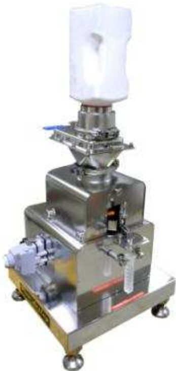
Filling of syringe for pharma industry: set point ~30 g, standard deviation < 0.02 g.
