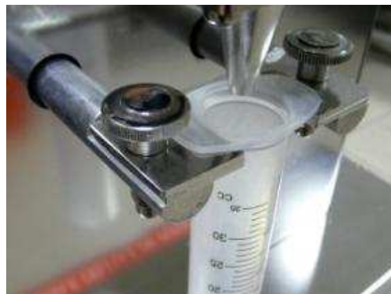
Filling of syringe for pharma industry: set point ~30 g, standard deviation < 0.02 g.
