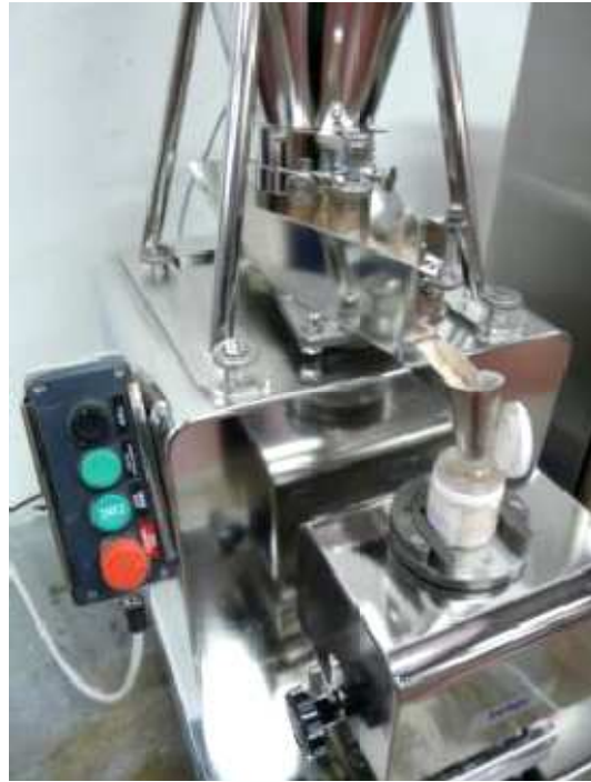
Feeling of pots, for pharmaceutical industry, the pot is laid manually on the balance.
