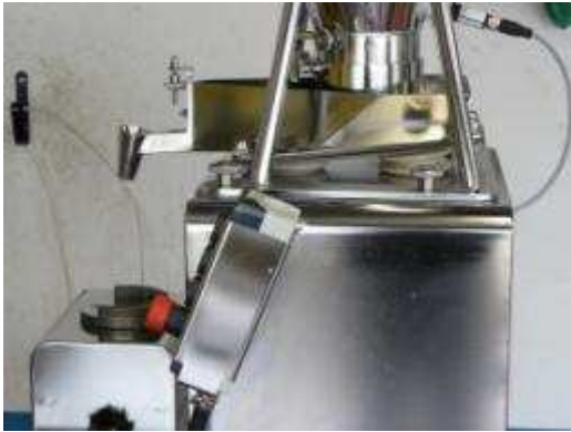
Feeling of pots, for pharmaceutical industry, the pot is laid manually on the balance.
